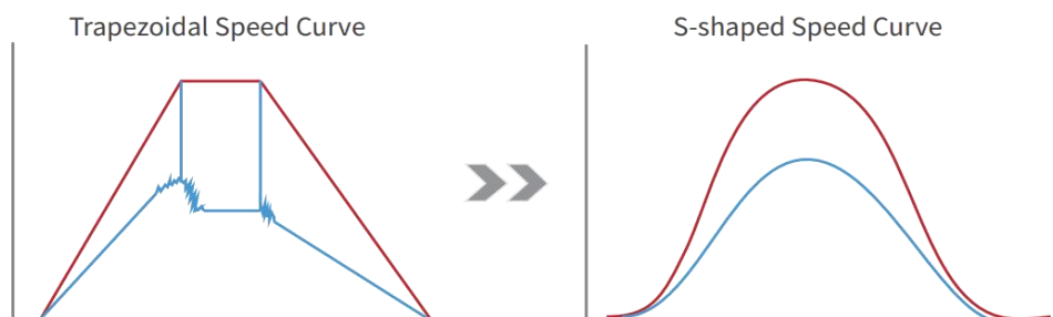
Figure 6-5 S-shaped speed step curve
